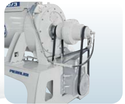
Detail of rotovariator and reduction gear
